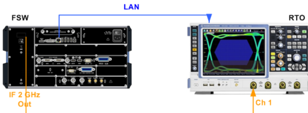
Figure 5-27: Measurement setup using the R&S FSW and an R&S RTO
