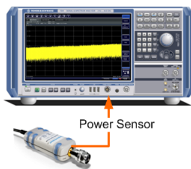
Figure 6-3: Connecting a power sensor using the POWER SENSOR interface
